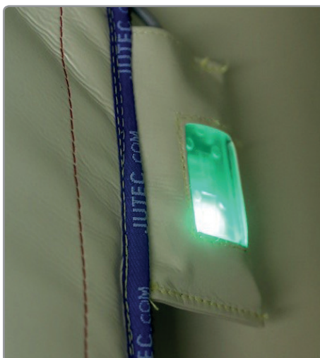
Status LED green - safety circuit closed.
