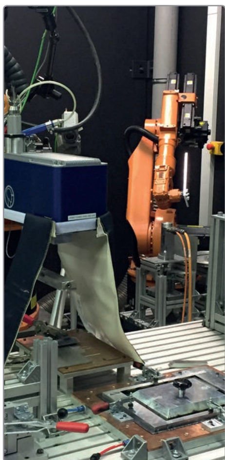
Guard against scattered radiation mounted on the scanning head.
