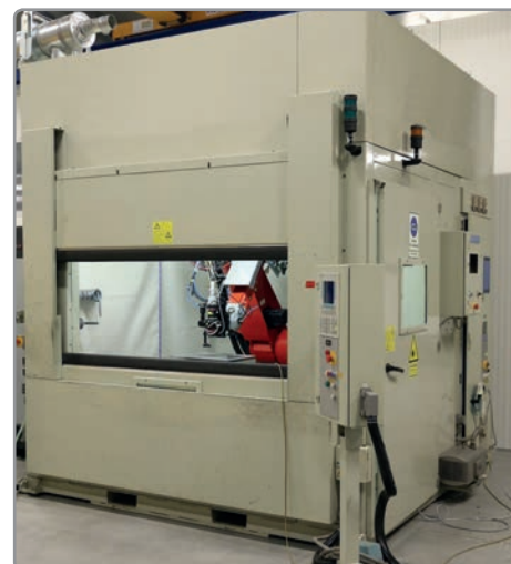
Robot cell, designed for low laser output. Thanks to the active laser protection system from JUTEC, it can now also be used for extremely high laser outputs and automated operation.
